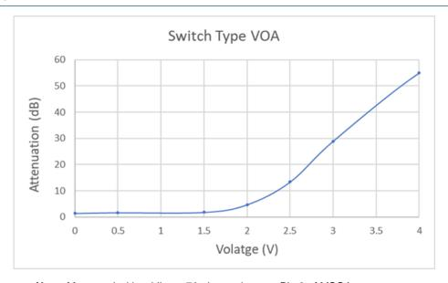
Note: Measured with adding a 70 ohm resistor on Pin 3 of MSOA.
